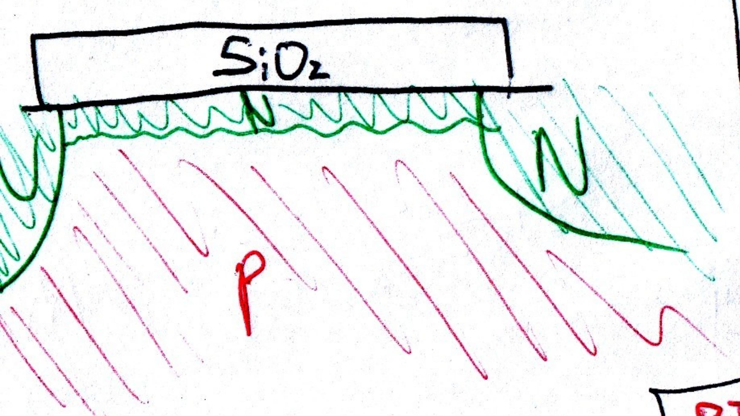
Since the oxide is non-conductive the electrons cluster around the gate, and in high enough concentrations, **REVERSE** the polarity of the silicon there.
