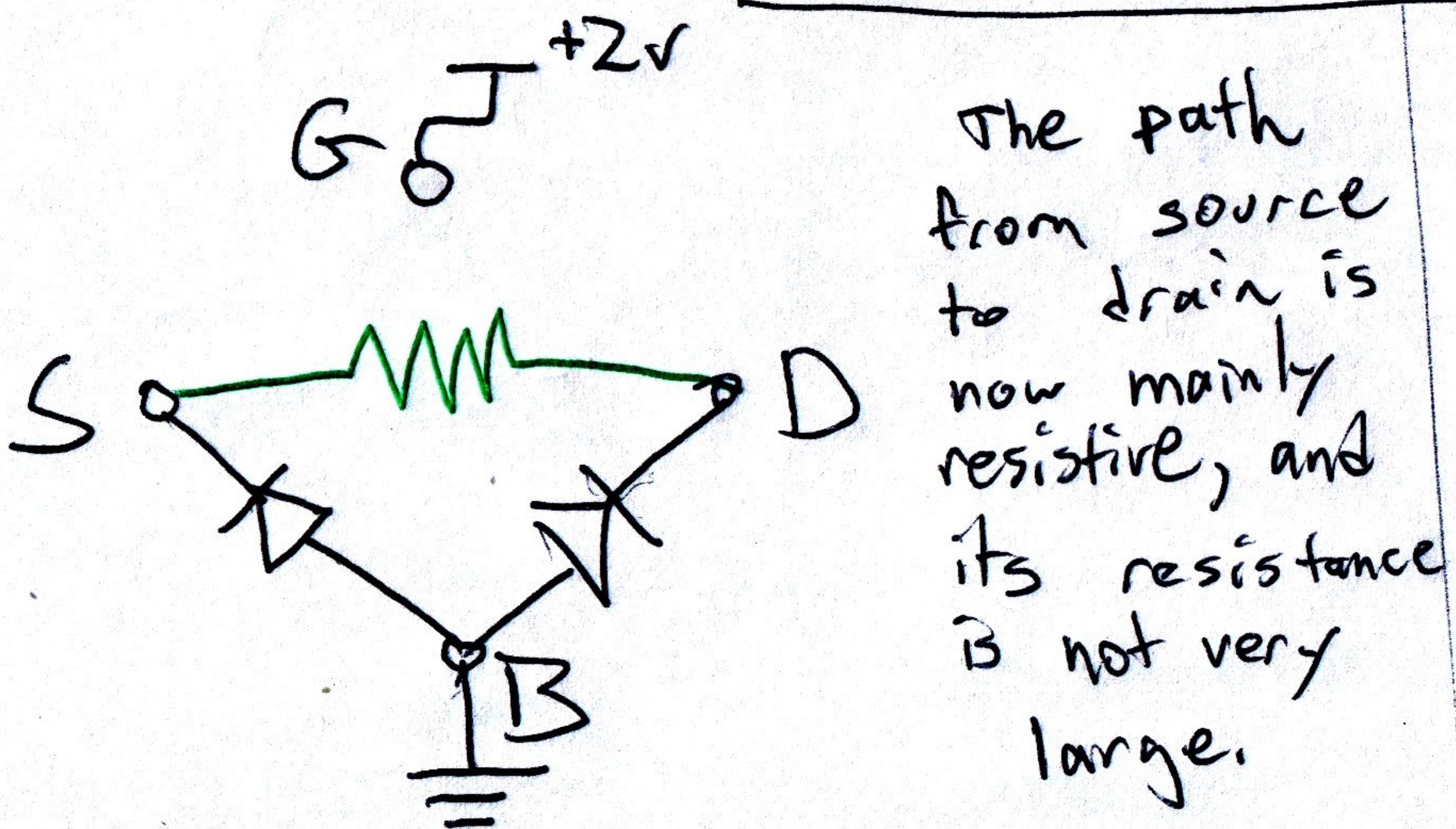
The path from source to drain is now mainly resistive, and its resistance is not very large.
