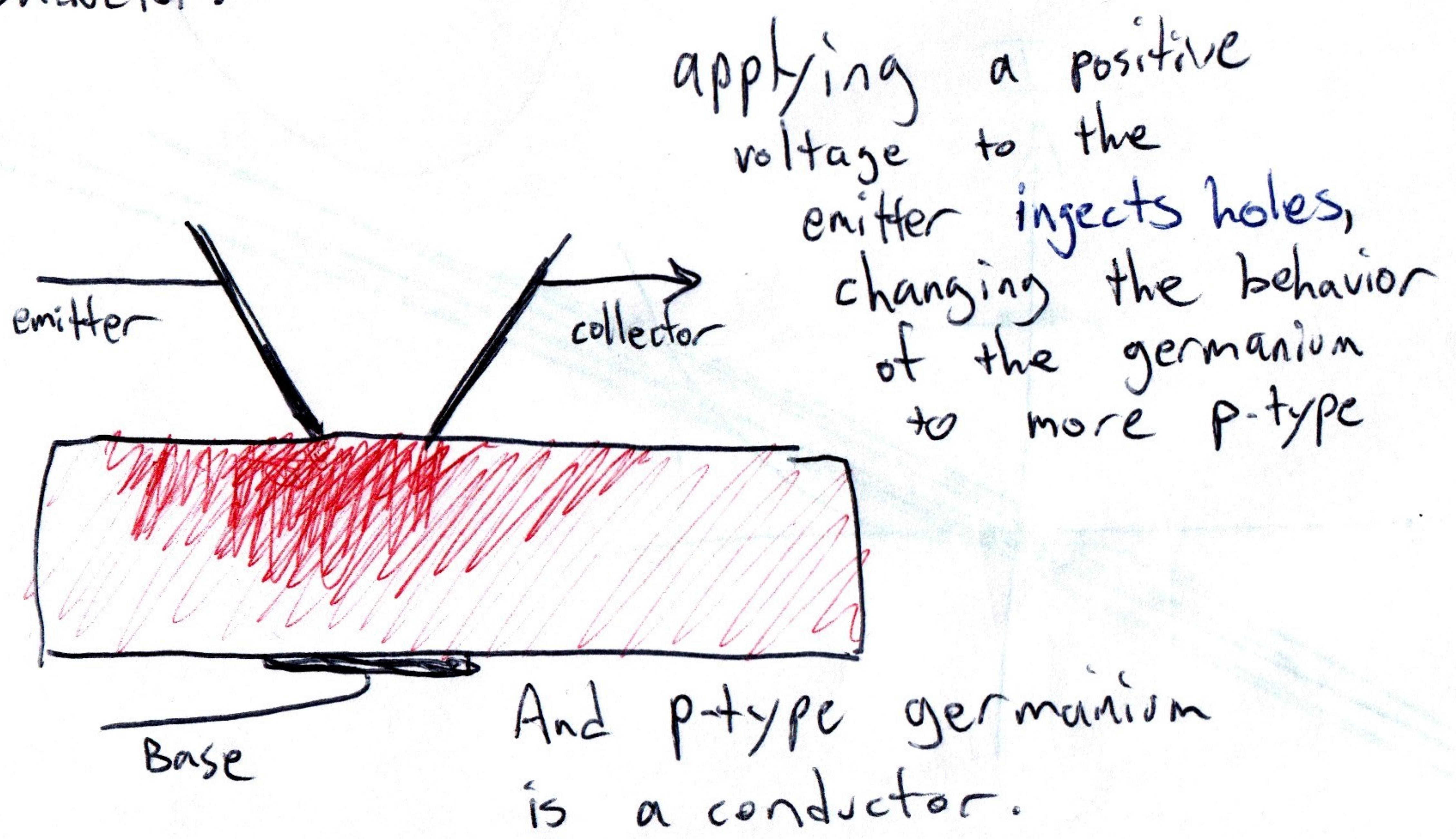
All but the most radically experimental transistor replacements work this way: by manipulating effective doping levels.
