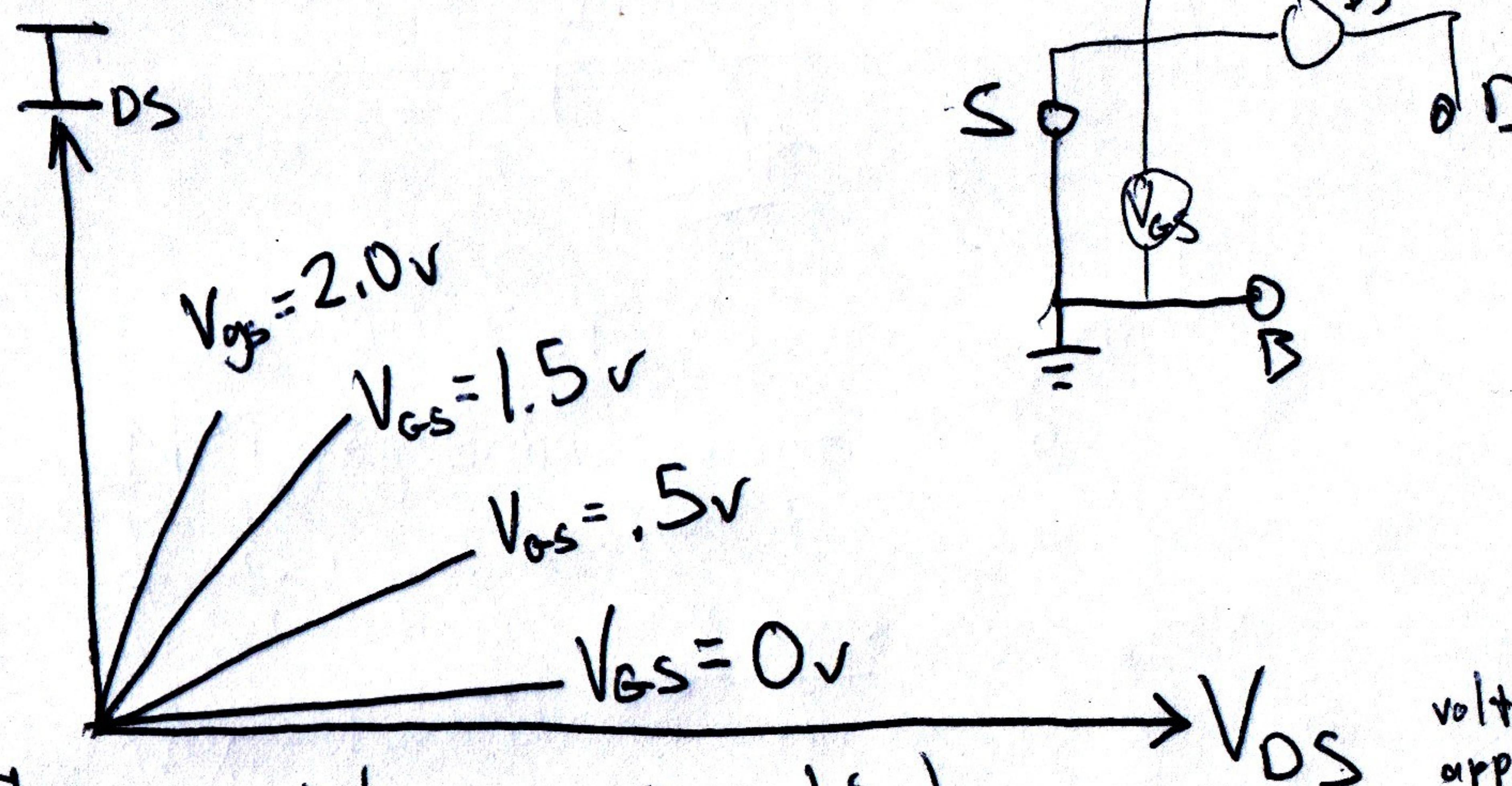
The resistance is high with no voltage on the gate, but at higher gate voltages, it is reduced.
